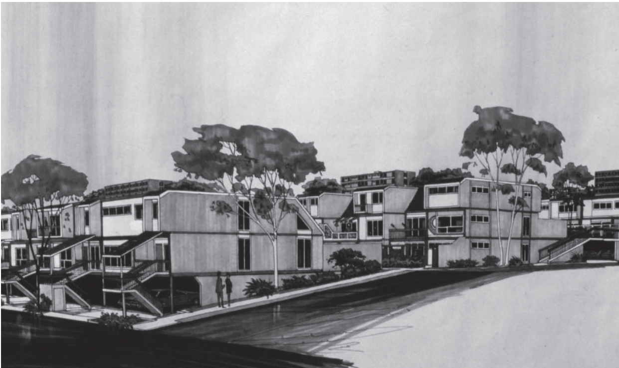
The Living System was a modular multifamily concept developed by Slayter Associates Inc., in the sixties in conjunction with Cornell University. It was designed from scratch to make the most of modular potential, rather than emulating residential architecture. Rendering by Dan Eacret, 1969
