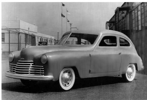
His dream was a postwar $400 car, something like an updated Model A. This fiberglass 1945 prototype was one of several he had built (with styling by engineers!).
